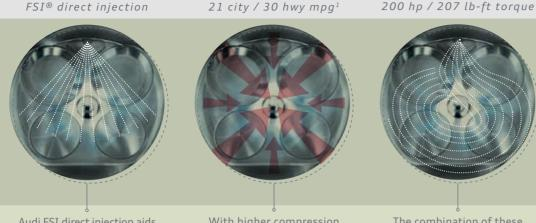
Audi FSI direct injection aids in cutting down on waste and increases power by delivering a precise amount of fuel directly into the combustion chamber, helping ensure a more complete combustion.
