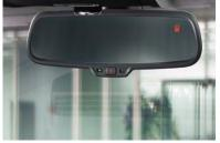
Auto-dimming interior rear view mirror with digital compass
