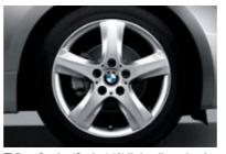
□ Star Spoke (Style 142) light alloy wheels with run-flat<sup>1</sup> all-season tires. In front:  $17 \times 7.0$  wheels and 205/50 tires; in back:  $17 \times 7.5$  wheels and 225/45 tires.<sup>3</sup> (No-cost opt. on 135i)
