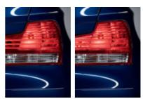
■ Adaptive Brake Lights increase vehicle visibility and signal the intensity of your braking action. In the event of an emergency stop, the illuminated area of the brake lights is increased, so traffic following behind you knows to stop quickly.
