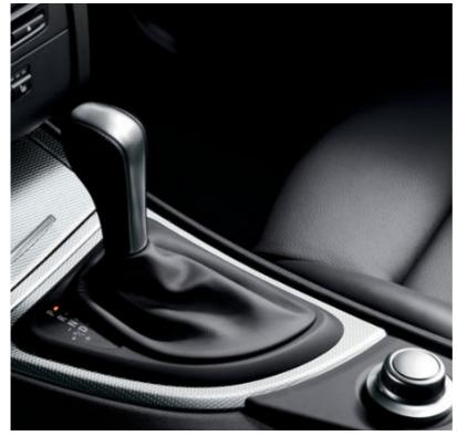
□ **6-speed STEPTRONIC automatic transmission** provides a choice of three modes: "Drive," which incorporates BMW's Adaptive Transmission Control; "Sport" automatic, for a more dynamic shift pattern; and STEPTRONIC automatic, for the hands-on control of a manual without using a clutch.
