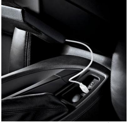
■ Auxiliary input port lets you connect an external audio source, such as an iPod<sup>®</sup> or MP3 player.
