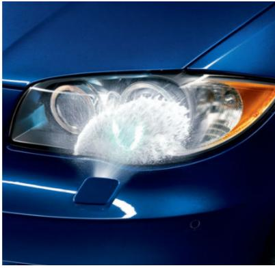
**High-intensity headlight washers** help keep lights clean of ice, mud, road salt and other coatings, for maximum road lighting and enhanced driving visibility. (Retractable headlight washers std. in 135i; headlight washers in the 128i Cold Weather Package are not retractable.)
