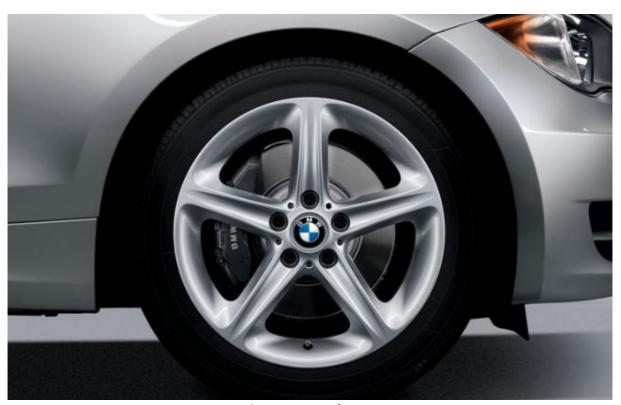
■ Star Spoke (Style 264) light alloy wheels and run-flat<sup>1</sup> performance tires.<sup>2</sup> In front: 18 x 7.5 wheels and 215/40 tires; in back: 18 x 8.5 wheels and 245/35 tires.<sup>3</sup> (std. on 135i)
