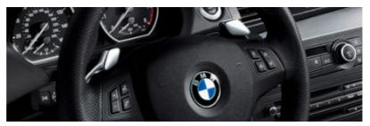
□ Steering wheel-mounted paddle shifters allow you to shift gears manually without a clutch. This optional feature comes included in the 1 Series Coupe when it is equipped with optional STEPTRONIC automatic transmission and Sport Package.
