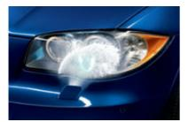
I / □ High-intensity headlight washers help keep lights clean of ice, mud, road salt and other coatings, for maximum road lighting and enhanced driving safety. (Retractable washers std. on 135i; fixed washers included in 128i Cold Weather Package. 135i shown)
