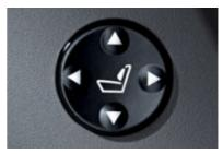
Lumbar support for front seats adds four-way power-adjustable comfort for the lower back. Lumbar support can be adjusted up/down and in/out.
