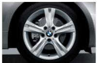
□ Star Spoke (Style 262) light alloy wheels and run-flat<sup>1</sup> performance tires.<sup>2</sup> In front:  $17 \times 7.0$  wheels and 205/50 tires; in back:  $17 \times 7.5$  wheels and 225/45 tires.<sup>3</sup> (included in 128i Sport Package)
