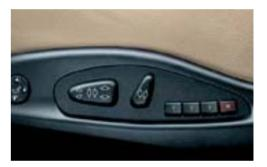
■ Power front seats include a driver's seat and mirror memory system, which lets up to three drivers set their preferred seat and exterior mirror positions. (Plus, the passenger's-side mirror tilts down when vehicle is shifted into reverse gear.) (Lumbar support shown standard in 330Ci; included in 325Ci Premium Package.)
