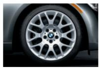
□ Cross Spoke (Style 197) light alloy wheels and run-flat¹ performance tires.² In front: 18 x 8.0 wheels and 225/40 tires; in back: 18 x 8.5 wheels and 255/35 tires. (included in 328i Sport Package)
