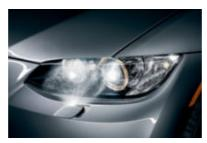
Retractable **high-intensity headlight washers** help keep lights clean of ice, mud, road salt and other coatings, for maximum road lighting and enhanced driving safety.
