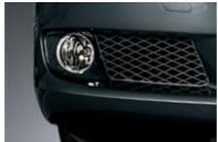
■ Halogen free-form foglights, integrated into the deep front spoiler, enhance your margin of safety in bad visibility. Ellipsoid free-form technology ensures even light distribution on the road.
