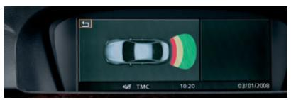
□ Park Distance Control uses ultrasonic sensors in the rear bumper to help you judge the distance to other cars and unseen objects when parking. The beeping becomes faster as your bumper approaches the object, turning into a constant tone when the distance is less than 12 inches.
