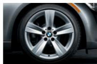
Star Spoke (Style 189) light alloy wheels and run-flat<sup>2</sup> performance tires.<sup>3</sup> In front: 18 x 8.0 wheels and 225/40 tires; in back: 18 x 8.5 wheels and 255/35 tires. (335i Sport Package)
