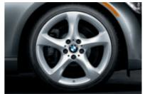
Star Spoke (Style 230) light alloy wheels and run-flat<sup>2</sup> performance tires.<sup>3</sup> In front: 19 x 8.0 wheels and 225/35 tires; in back: 19 x 9.0 wheels and 255/30 tires.
