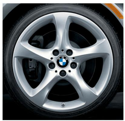
$\square$  Star Spoke (Style 230) light alloy wheels and run-flat performance tires.<sup>2</sup> In front: 19 x 8.0 wheels and 225/35 tires; in back: 19 x 9.0 wheels and 255/30 tires.<sup>3</sup> (opt. on 335i, requires optional Sport Package)
