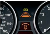
☐ Active Cruise Control system uses radar measurements to automatically maintain a pre-set speed and distance between your vehicle and the one ahead in highway driving.¹ (requires automatic or Sport Automatic transmission)
