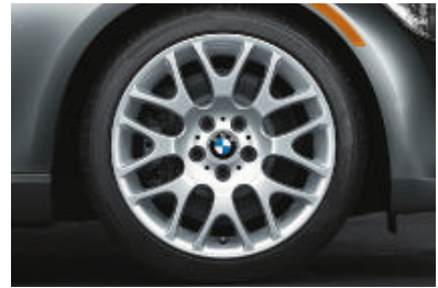
Cross Spoke (Style 197) light alloy wheels and run-flat 2 performance tires. 3 In front: 18 x 8.0 wheels and 225/40 tires; in back: 18 x 8.5 wheels and 255/35 tires. (328i Sport Package)
