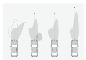
Adaptive Headlights create cones of light that follow the direction of the headlights. Cornering Lights illuminate the side of the road when turning, helping to reveal obstacles, cyclists and pedestrians.
