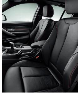
Ten-way adjustable front sport seats make the driving experience more enjoyable with adjustments for forelaft, seat height, backrest angle, seat angle and thigh support. Side bolsters can be power-adjusted to comfortably fit your back while helping to hold you firmly in place during cornering. Includes two-way headrests with Active Head Restraints feature.
