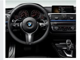
Leather-wrapped multi-function M sport steering wheel has a smaller diameter and a thicker rim for enhanced grip. The speedometer and tachometer come with a contrasting red surround.
