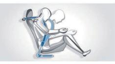
three-point safety belts, automatic safety-belt pretensioners, seat bolsters that help prevent occupants from sliding forward, and Active Head Restraints. This system helps provide optimum restraint in a collision.
