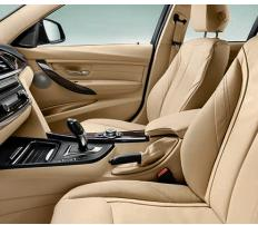
Power front seats, shown here with Venetian Beige Dakota Leather with exclusive stitching, offer eight-way adjustment including two-way adjustment of headrests. The driver's seat provides individual adjustments for seat height and backrest, fore and aft position and seat angle.
