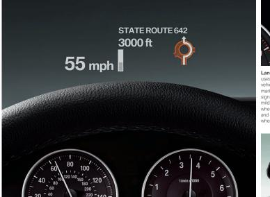
Head-up Display projects important travel information, such as vehicle speed and Check Control warnings, onto the windshield directly in your field of vision. Data is shown in full color, making information even more precise and easier to process. Additional information, including Lane Departure Warning messages and Navigation directional arrows and instructions, can also be displayed.
