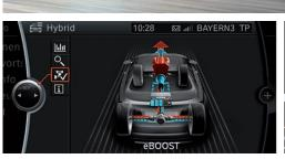
Boost function: when required, energy from the high-performance battery is used to enable a short-term boost of power. A benefit of this technology is strong and immediate power delivery.
