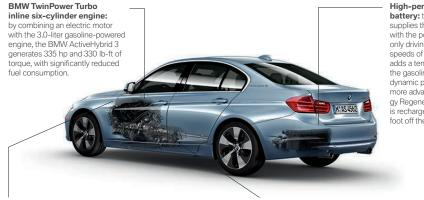
High-performance lithium-ion battery: this highly efficient battery supplies the BMW ActiveHybrid 3 with the power needed for electriconly driving for 2-2.5 miles at speeds of up to 37 mph. It also adds a temporary 55-hp boost to the gasoline engine for increased dynamic performance. Using a more advanced form of Brake Energy Regeneration, this storage unit is recharged whenever you lift your foot off the accelerator pedal.
