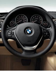
Three-spoke, leather-wrapped multi-function sport steering wheel with manual tilt/telescoping feature lets you keep both hands on the wheel while adjusting both the audio and a Bluetooth® enabled mobile phone, if so equipped. Voice command (included with Navigation system) can be used to change audio selections, Navigation system destinations and telephone entries.
