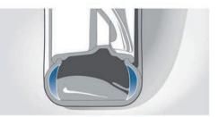
their shape and rim position even after suffering a complete loss of tire pressure. They allow you to continue driving at a reduced speed until you reach a safe area to change a tire or wait for Roadside Assistance. The Tire Pressure Monitor alerts you when there is a drop in tire pressure; if the loss is severe, an acoustic warning is triggered.
