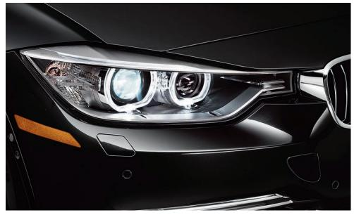
Xenon Adaptive Headlights optimize road illumination when entering a turn or corner, helping to enhance visibility when driving at night. Sensors continuously monitor the angle of the steering wheel to determine the direction in which your vehicle is heading. The outer headlights swivel accordingly, up to 15 degrees left or right.
