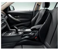
Power front seats, shown here with Black Dakota Leather with Dark Oyster highlight piping, offer eight-way power adjustment plus two-way manual headrest adjustment. The driver's seat provides individual adjustments for seat height and backrest, fore and aft position and seat angle.
