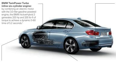
High-performance lithium-ion battery: this highly efficient battery supplies the BMW ActiveHybrid 3 with the power needed for electriconly driving for up to 2.5 miles at speeds of up to 47 mph in ECO PRO mode. It also adds a temporary 55-hp boost to the gasoline engine for even greater dynamic performance. Using an advanced form of Brake Energy Regeneration, this storage unit is recharged whenever you lift your foot off the accelerator pedal.
