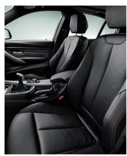
12-way power front sport seats make the driving experience more enjoyable with adjustments for forefaft, seat height, backrest angle, seat angle and thigh support. Side bolsters can be power-adjusted to comfortably fit your back while helping to hold you firmly in place during cornering. Includes two-way headrests with Active Head Restraints feature.
