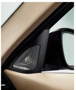
Harman Kardon® Surround Sound System is a 16-speaker, multi-channel system that outputs reproduction of the surround information contained in the stereo signal in a nine-channel format as well as 5.1 surround sound from a DVD source. Includes a powerful 600-watt digital amplifier with nine channels. The system compensates for driving noise in smooth steps with speed-dependent equalizing.
