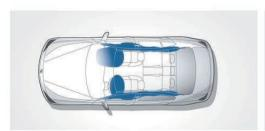
(SRS) determines which airbag(s) to deploy for optimal protection. When a safety belt is used, airbags deploy only at a higher crash severity; the force of the deployment depends upon the severity of the impact. Eight airbags offer specific protection: front airbags with advanced technology for driver and front passenger, front knee airbags, front-seat-mounted sideimpact airbags, and HPS (Head Protection System) bags for front and rear.
