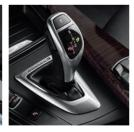
8-speed automatic transmission gear selector lever features an aluminum surround with special ActiveHvbrid 3 signature.
