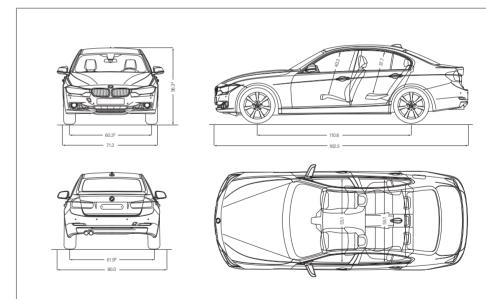
All dimensions in the technical drawings are shown, in inches, for 328i; dimensions for other models, if different, are footnoted.
