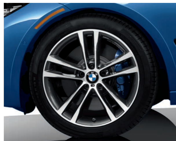
Double Spoke light alloy wheels (Style 598M) 19 x 8.0 front, 19 x 9.0 rear; and 225/45 front, 255/40 rear run-flat 1 summer tires 2,3
