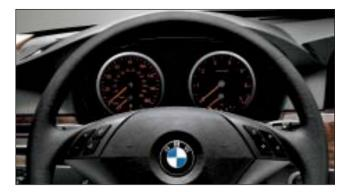
Primary gauges are recessed under a cowl, and designed for glare-free vision during the day. At night, the gauges glow in a color that is restful on the eyes.
