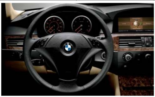
■ 3-spoke leather-wrapped multi-function steering wheel lets you keep both hands on the wheel while adjusting various comfort functions, such as changing the radio, CD selections and volume. Optional Voice Control (included with optional on-board navigation system) can be used to change radio stations and audio selection, navigation system destinations, and (accessory) telephone entries.
