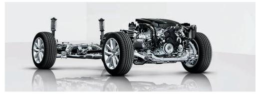
Integral Active Steering, in rear-wheel-drive vehicles, delivers more direct response with a small turn of the steering wheel at speeds of up to 30 mph. This feature also steers the rear wheels up to 2.5 degrees in the opposite direction, giving the effect of a shortened wheelbase for enhanced maneuverability. When changing lanes at speeds over 50 mph, both front and rear wheels turn in the same direction, giving the feel of an extended wheelbase.
