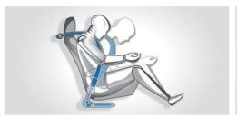
BMW restraint system for driver and front passenger combines threepoint safety belts, automatic safety-belt pretensioners, and seat bolsters that help prevent occupants from sliding forward. Active Head Restraints in the front seats reduce the risk of whiplash or neck/head/spine injury. When sensors detect a rear-end collision, the headrests automatically and rapidly pivot forward, supporting the occupant's heads.
