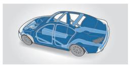
**Body stiffness.** The intelligent use of high-strength multi-phase steel and aluminum provides a high degree of body stiffness and crash resistance. Components, such as the A-pillars and windshield frame, include special reinforcements to provide optimum occupant protection.
