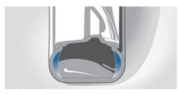
Run-flat tires. Thanks to reinforced sidewalls, run-flat tires maintain their shape and rim position even after suffering a complete loss of tire pressure. They allow you to continue driving at a reduced speed until you reach a safe area to change a tire or wait for Roadside Assistance. The Tire Pressure Monitor alerts you when there is a sudden and irregular drop in tire pressure. Should the target pressure of a tire fall below 25 percent, both a warning light and acoustic alarm are triggered.
