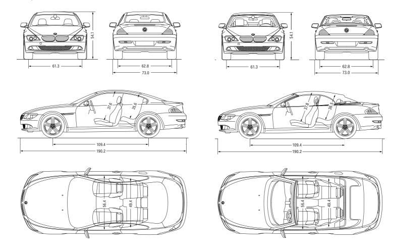
All dimensions are shown in inches and apply to models with standard wheels. NOTE: Measurements do not include vehicle width from mirror to mirror.
