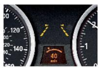
□ Lane Departure Warning feature<sup>2</sup> alerts the driver by discreetly vibrating the steering wheel if the vehicle crosses lane markings without using the directional signal.
