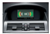
■ Park Distance Control (PDC), front and rear, helps parking and maneuvering in tight spaces. The distance between your vehicle and an obstacle is indicated by an acoustic signal that increases in intensity as your bumper approaches the object, turning into a constant tone when the distance closes to 12 inches. A visual representation is also projected on the iDrive Control display.
