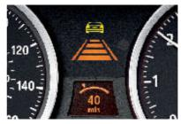
□ Active Cruise Control (ACC) with Stop & Go allows the driver to preset a desired speed. When ACC recognizes slower-moving vehicles ahead, it automatically brakes to maintain a preset distance, then resumes the set speed as soon as possible.¹ In traffic, Stop & Go can reduce the speed down to a standstill. (requires optional Sport Automatic transmission)
