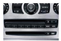
■ Six programmable memory keys offer convenient storage of your most frequently accessed iDrive settings, such as favorite radio stations, Navigation system addresses, phone numbers and more.
