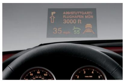
□ Head-up Display projects important travel information, such as current speed, on the windshield directly in the driver's line of vision. Directional arrows from the Navigation system, Check Control data and optional Active Cruise Control<sup>3</sup> functions can also be displayed. (note: Head-up Display not available with green band windshield)
