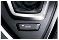
■ Dynamic Driving Control (Sport button), when activated, quickens the vehicle's response and performance for more dynamic steering, acceleration and gear shift changes.
