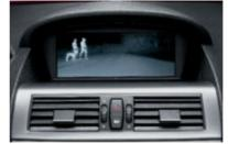
□ Night Vision is BMW's amazing system that lets you see pedestrians or animals in the dark – up to 1640 feet ahead. Using an infrared camera built into the front of the vehicle, you will be able to see potential road hazards displayed on your Navigation system monitor, and avoid them well before they are visible to the naked eye. At higher speeds, a digital zoom provides enlarged images of more distant objects on the screen.
