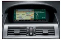
■ Navigation system covers the U.S. with a single DVD. Accessed via Voice Activation or through the iDrive Controller, the Navigation system uses GPS satellites and DVD technology to create a map of your area on the glare-free dash monitor. The system shows – and tells – the direction to your desired destination; it also provides Real Time Traffic Information on potential traffic problems and solutions.
