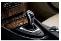
☐ 6-speed Sport Automatic transmission provides extremely fast synchronized shifting, whether performed by the automatic shift mode or by means of the Formula 1-inspired steering wheel-mounted paddle shifters. (no-cost option)
