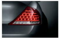
■ Adaptive Brake Lights help following drivers judge your braking intensity. Under light braking, the lower three rows of long-life LEDs in the rear brake-light unit illuminate. During panic braking, Dynamic Brake Control (DBC) signals for the two upper rows of LEDs to illuminate. For 2008, the brake-light strip on the trunk (not shown) has been made wider and moved to the top of the spoiler lip.
