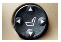
■ Four-way power lumbar support for front seats offers comfort and lower back muscle support. Lumbar support can be adjusted four ways: up/down and in/out.
