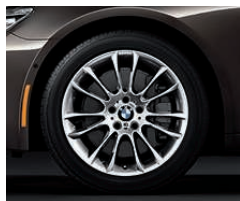
V Spoke (Style 302M) 19 x 8.5 front, 19 x 9.5 rear light alloy wheels with 245/45 front, 275/40 rear run-flat 1 performance tires . 2,3 Also: 19 x 8.5 light alloy wheels with 245/45 run-flat 1 all-season tires. 2
