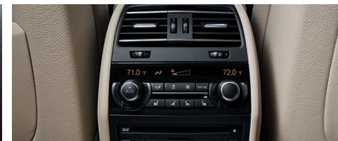
Four-zone automatic air conditioning delivers draft-free ventilation. In front, automatic climate control includes fully separate left/right controls, solar sensor, automatic recirculation, and heat-at-rest feature. The rear cabin offers left/right temperature-controlled outlets and auto ventilation.
