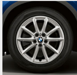
■ 17" light alloy V-spoke style 560 wheels, Reflex Silver, 7.5J x 17 with 225/55 R17 tyres. 1
