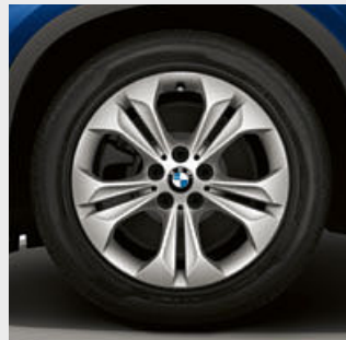
□ 17" light alloy Double-spoke style 564 wheels, Reflex Silver, 7.5J x 17 with 225/55 R17 tyres.
