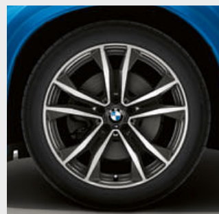
■ 19" M light alloy Double-spoke style 715 M wheels, Orbit Grey, 8J x 19 with 225/45 R19 run-flat tyres. 4
