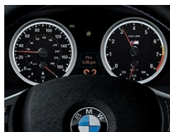
M instrument cluster with circular speedometer and rev counter (with variable red line), plus fuel and oil temperature gauges.
