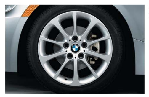
■ 17 x 8.0 Turbine (Style 200) lightalloy wheels and 225/45R-17 run-flat<sup>1</sup> performance tires.<sup>2</sup> (Z4 Coupe 3.0si)
