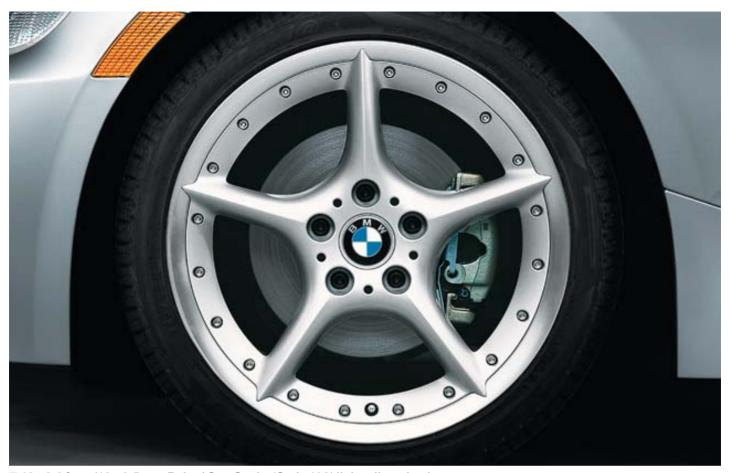
$\square$  18 x 8.0 front/18 x 8.5 rear Bolted Star Spoke (Style 108) light-alloy wheels and 225/40R-18 front, 255/35R-18 rear run-flat<sup>1</sup> performance tires.<sup>2</sup> (included in optional Z4 Roadster 3.0si Sport Package)
