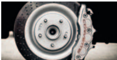
Silver calipers 1 shown with larger cross-drilled brake rotors for 427 Convertible, Z06 and Grand Sport.
