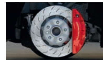
Red calipers standard on Z06 and available on Stingray and Grand Sport (Brembo slotted brakes included with available Z51 Performance Package shown)
