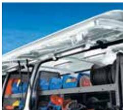
**Available Access Packages:** These packages offer easy interior access to tools and cargo. Each includes three exterior, remote-release, side-access panels that can be opened by Remote Keyless Entry. Not available with optional driver-side 60/40 swing-out doors or sliding passenger-side door.
