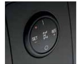
Power takeoff (PTO) capability<sup>6</sup> allows HD Chassis Cab, with the available Duramax 6.6L Turbo-Diesel V8 engine, to power auxiliary equipment like a dump body or hydraulic motors for generators and tools. This feature runs off the available Allison 1000 Series 6-speed automatic transmission.
