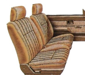
Cloth and vinyl reclining bucket seats with adjustable head restraints are standard.
