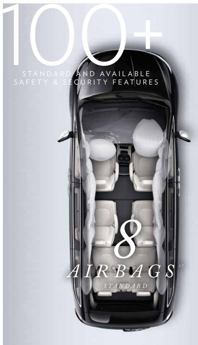
**Equipped to Protect** The standard air bags<sup>17</sup> include advanced multistage front air bags<sup>17</sup> with adaptive venting technology, front occupant knee air bags<sup>17</sup> supplemental front-seat-mounted side-impact air bags<sup>17</sup> and side-curtain air bags<sup>17</sup> which extend over all three outside seating rows.
