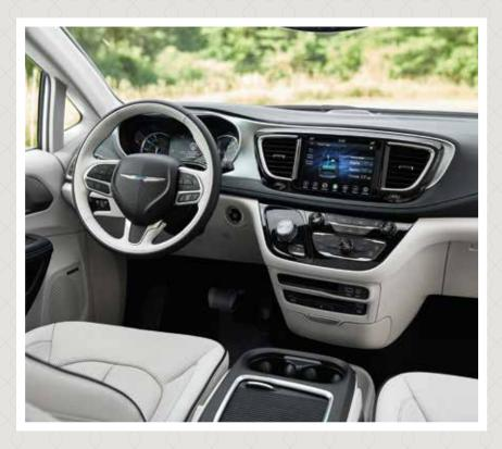
Monitoring the energy input and output is so simple, you'll never second-guess your power source. The standard Uconnect® 8.4-inch touchscreen system with available navigation and voice command includes Hybrid Electric Pages providing vehicle information screens for Power Flow, Driving History and Charge Scheduling.
