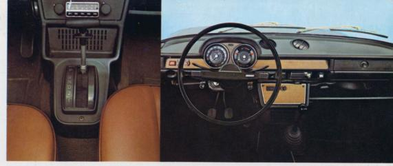
Automatic transmission is available as an option on the FIAT 124 Special and Station Wagon. The unit is a precision torque converter with 3-speed planetary gear set designed expressly for efficient FIAT engines.
