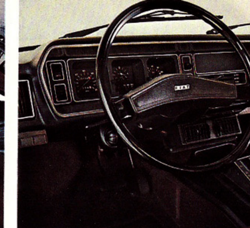
Trip odometer, electronic tachometer, quartz crystal electric clock — they're all standard on the dashboards of all three FIAT 131 models.
