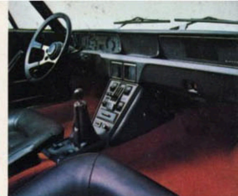
The action starts here: five precision instruments are mounted in the dash panel; all switches and the stick are close at hand in the full-length console.
