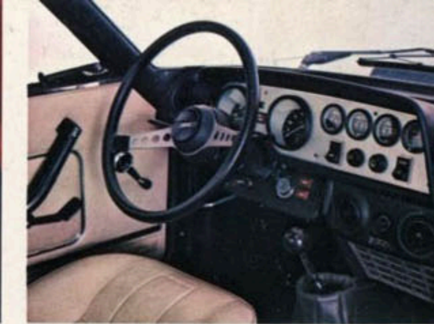
From left to right: speedometer with trip recording odometer; electronic tachometer; fuel gauge; oil pressure gauge; temperature gauge; quartz crystal electric clock.
