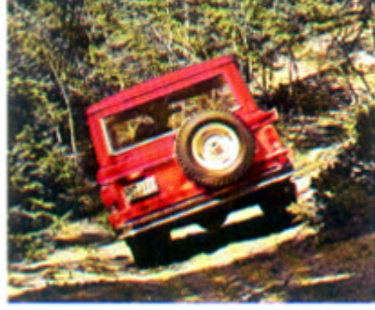
Slope-hugging stability. Bronco has the optimum track width. Wheels are set wide apart for excellent off-road stability, yet narrow enough to negotiate twisting paths and trails. And Bronco's "identical track" front and rear axles allow the rear wheels to follow in the same path made by the front wheels for easier trailblazing.
