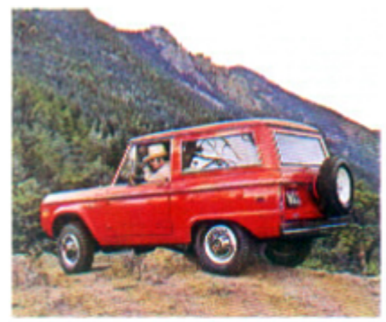
Excellent ground clearance. Bronco combines the best ground clearance amidships (w/optional 6.50 x 16 tires) with a big ramp breakover angle to allow crossing over high projections. Bronco's excellent angles of approach and departure provide greater freedom from hangups when approaching or leaving steep inclines and ditches.
