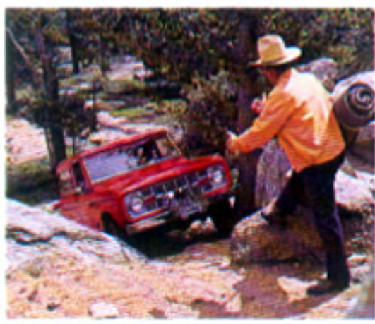
Superior maneuverability. Maneuvering around boulders and other off-road obstacles is a cinch with a nimble Bronco. Wide-track front axle with 37° turn angle provides best maneuverability of any 4-wheeler. Bronco can turn in a small 33.6-foot circle—tree to tree—sharper than anything in its class.
