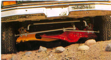
Twin-Traction Beam independent front suspension.
