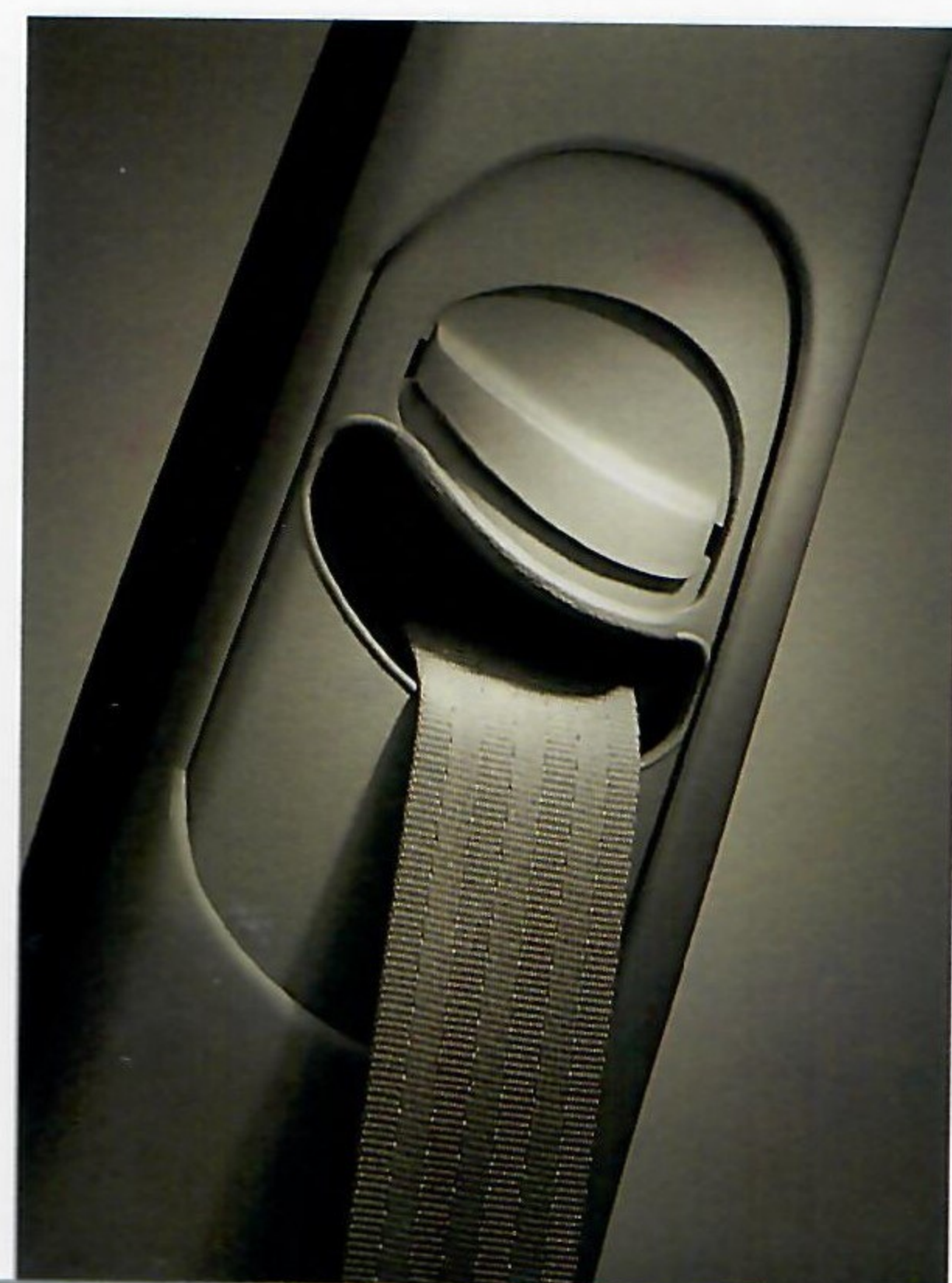
The shoulder belts have D-ring height adjusters to satisfy the comfort needs of short and tall people alike.
