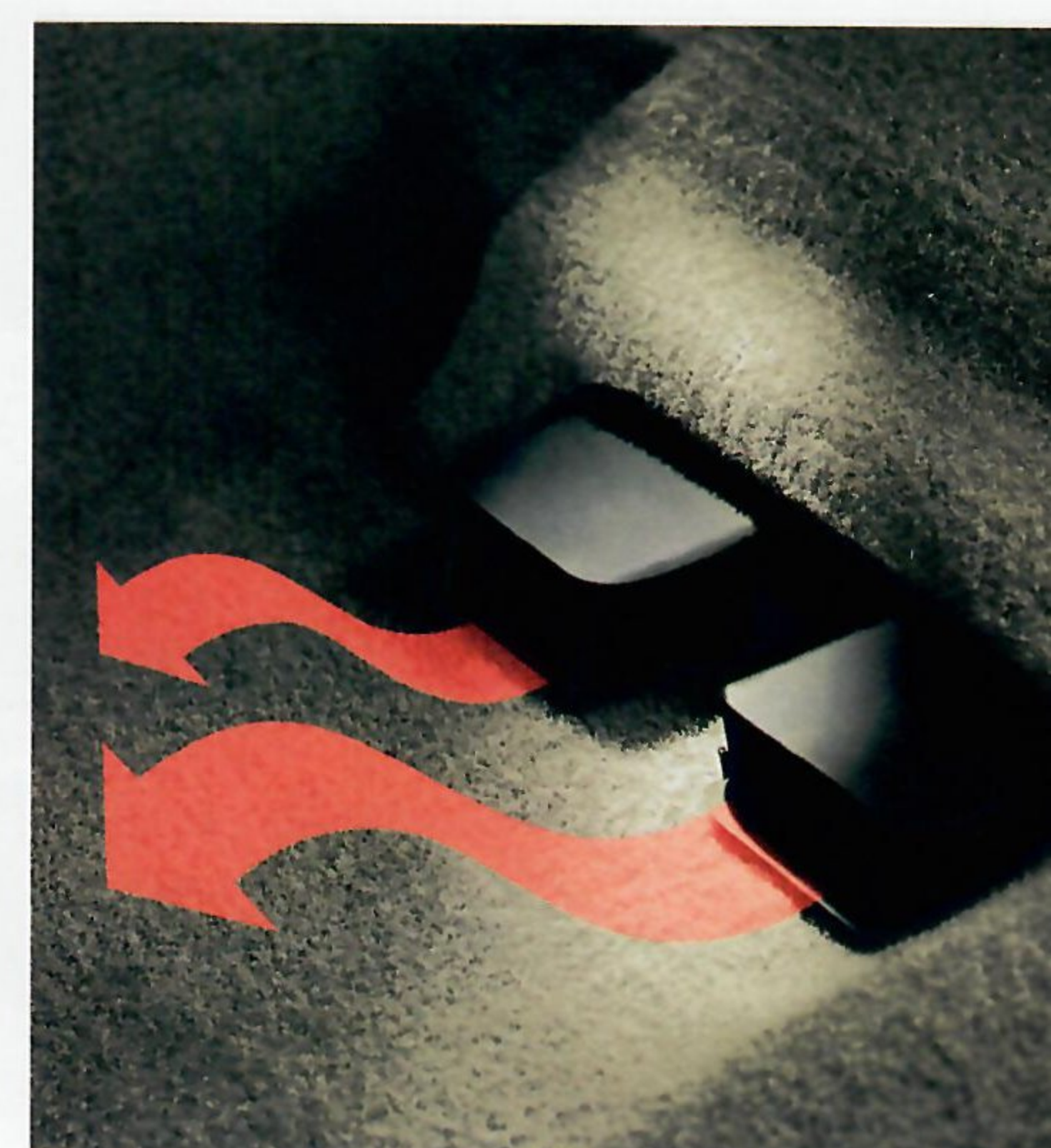
Heat is distributed through vents on the instrument panel and also through rear seat area ducts.
