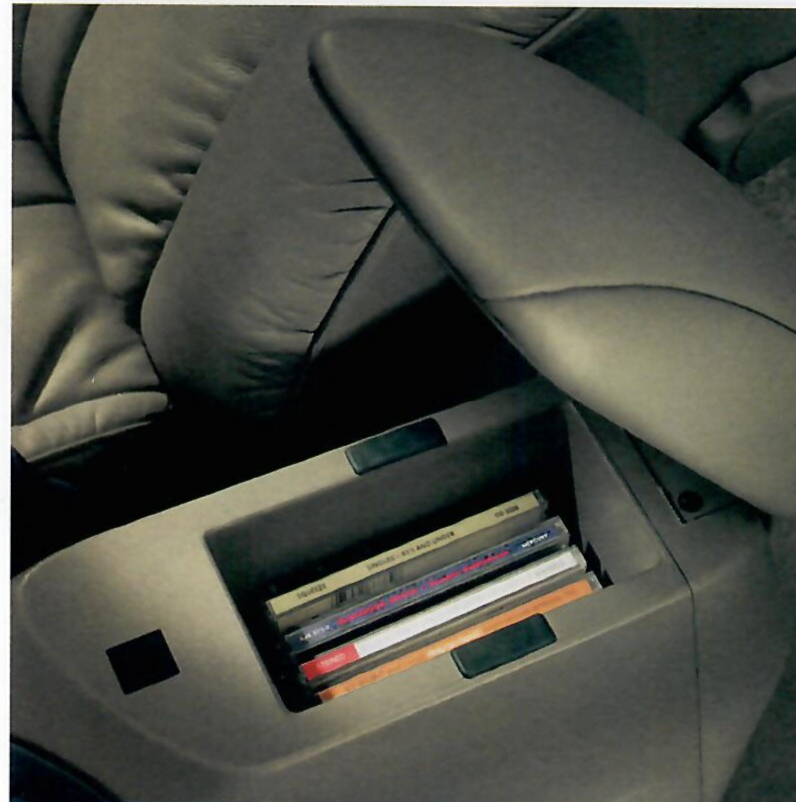
In the full-length center floor console in Contour LX and SE are slots for tape cassettes and compact discs.
