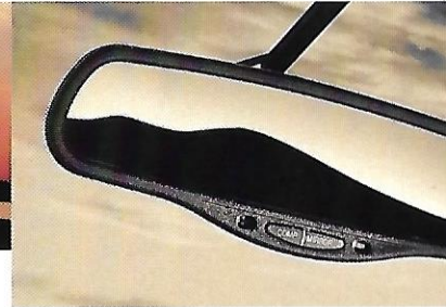
An automatic dimming rearview mirror, which includes a heated element, is part of the optional LX Comfort Group.
