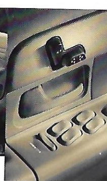
Power windows and door lock are standard. The "express-down" feature allows the driver's window to be lowered completely with just one touch of
