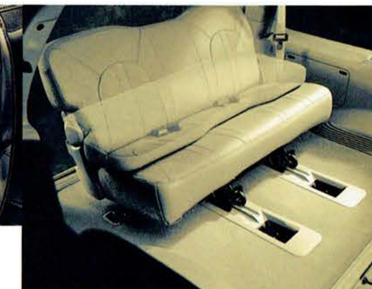
Versatile fold-flat third-row bench seat with rollers allows for easy installation and removal.
