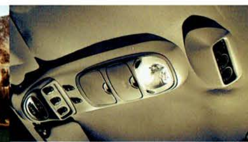
Standard overhead console includes map lights, power rear quarter window switches, electronic display, sunglasses holder, and a bin for a garage door opener.
