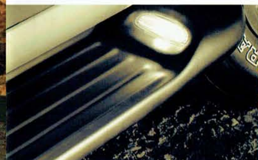
Standard running boards provide easy access and are illuminated for excellent visibility.
