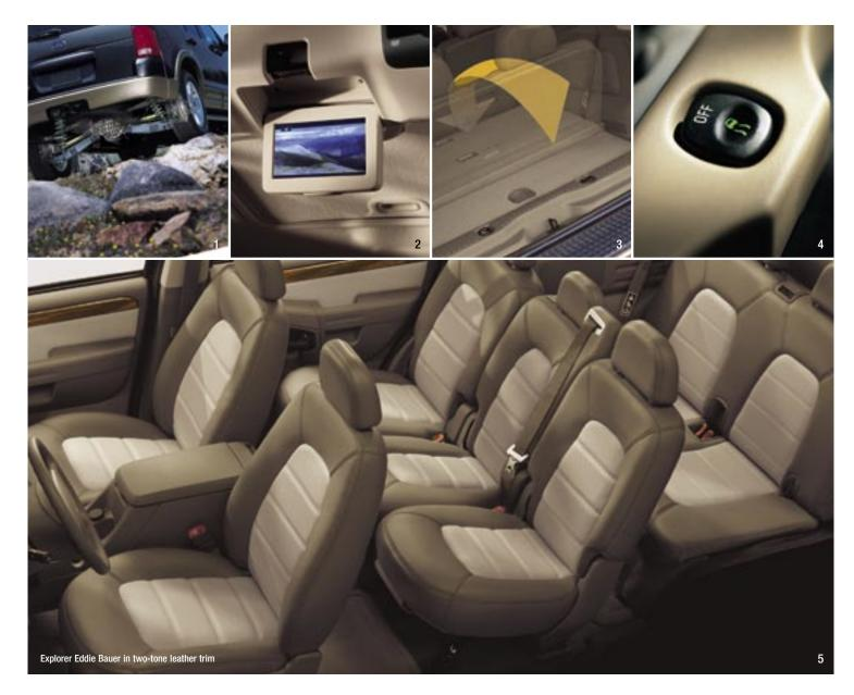
■ Explorer's Independent Rear Suspension allows each wheel to move independently of the other, resulting in a smooth ride. 2 The available Rear Seat DVD Entertainment System includes a fold-down 7" LCD screen, two sets of wireless headphones and a remote control. I The easiest and fastest folding available third-row seat disappears into the
