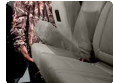
NEW SUPERCREW ONE-TOUCH 60/40 SPLIT REAR SEAT has mechanically assisted seat bottoms that easily and securely fold up against the back of the cab.
