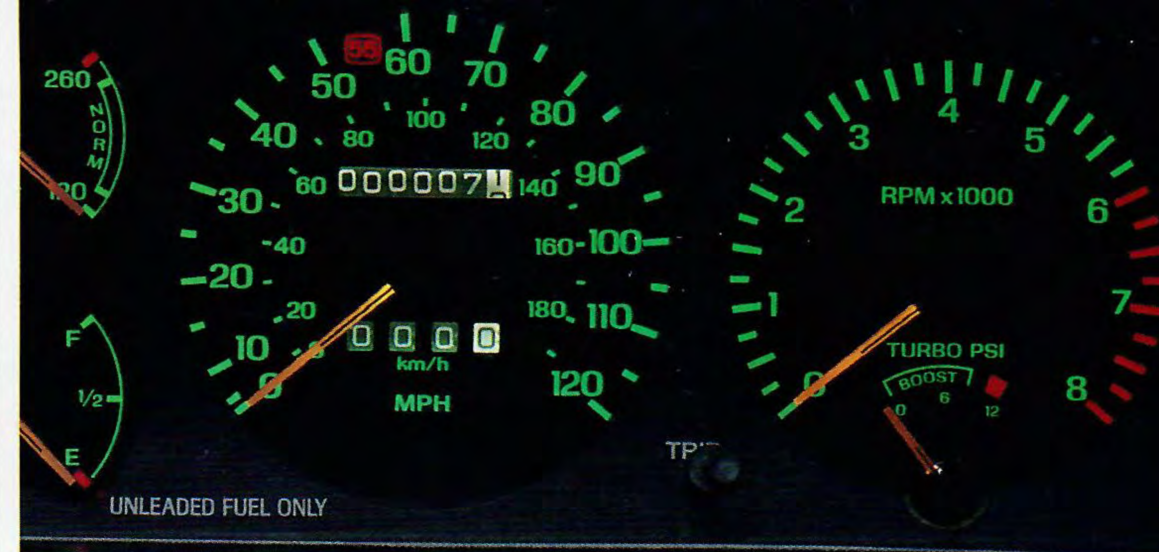
A turbo boost gauge is added to Probe's standard package of analog gauges. Also a GT feature is a low oil level warning light.
