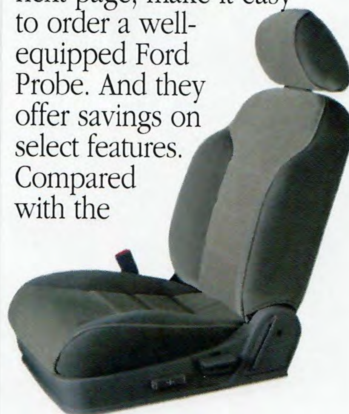
The power driver's seat, optional in LX and GT, provides forward/back and vertical height adjustment at the touch of a button.
