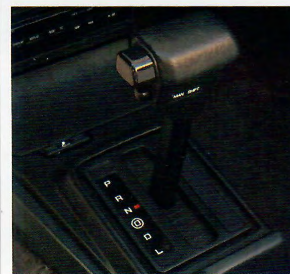
Electronically controlled, the optional 4-speed automatic transaxle is smooth and precise. The flexible Manual Shift mode permits selective shifting in first, second and third gears.
