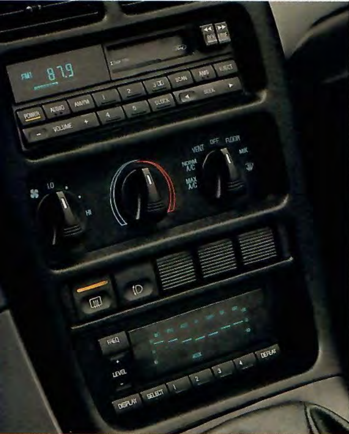
On the center panel console are heating/cooling, stereo system and other controls. As you can see in the photograph at right, this console is angled toward the driver, an important ergonomic design feature.
