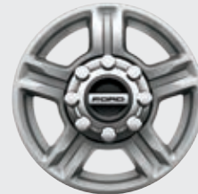
17" Cast-Aluminum with Bright Center Cap Optional: XL F-350 SRW Standard: XLT F-350 SRW
