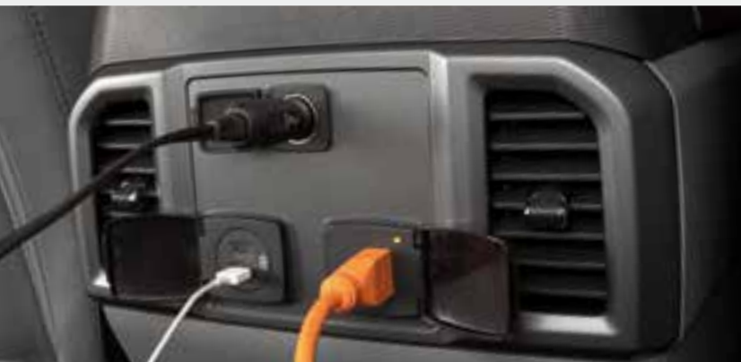
100V/400W AC POWER OUTLET ON CENTER CONSOLE REAR (SuperCab/Crew Cab) Standard on LARIAT; Available on XLT
