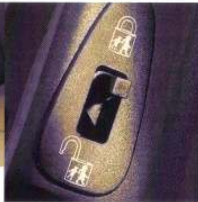
When activated, standard "childproof" rear door locks prevent doors from being opened from inside the vehicle.
