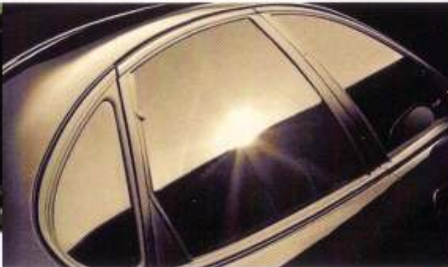
Standard solar tinted glass reduces heat build-up and helps the air conditioner cool the car faster.
