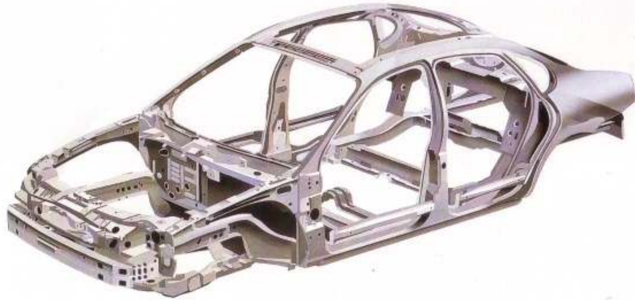
A high level of safety and durability has been achieved by means of a safety cell structural design.
