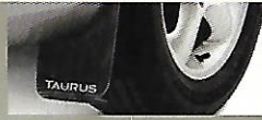
Splash Guards protect lower body panels from stones and other road debris.
