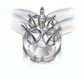
The 4-valve-per-cylinder design of every Civic engine allows a higher volume of fuel and air into the combustion chamber, helping it create more power and operate more efficiently at all rpm.
