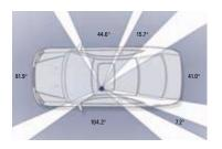
Honda engineers understand the importance of excellent outward vision, so they designed the new Civic with 294.6° of visibility to minimize blind spots for the driver.
