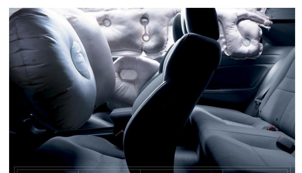
pretensioner seat belts An automatic seat-belt tensioning system helps hold the front-seat occupants securely in a collision. The system is triggered by the same sensors that deploy the airbags.
