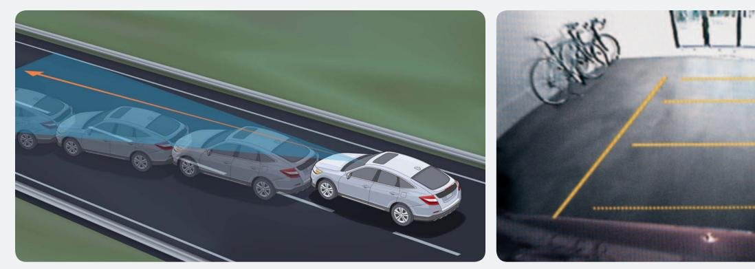
With the Lane Departure Warning (LDW)<sup>8</sup> system, a small camera between the windshield and the rearview mirror can track lane markings on the road. The system alerts you when it detects you moving into a different lane without signaling (EX-L models).
