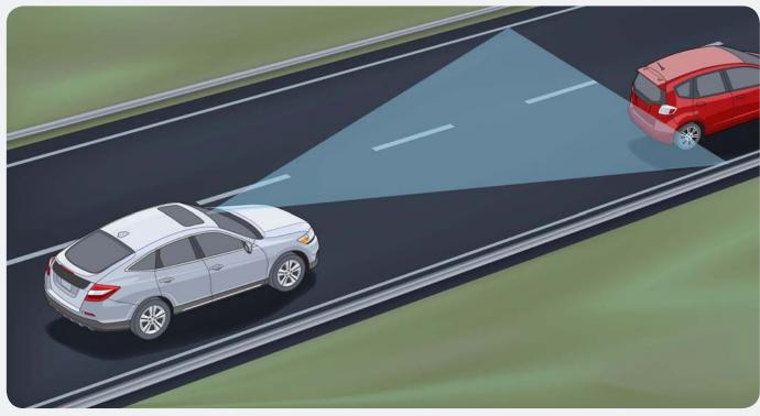
The Forward Collision Warning (FCW)<sup>7</sup> system can sense the presence of vehicles in front of you and issues alerts if it calculates that you are at risk of a collision (EX-L models).
