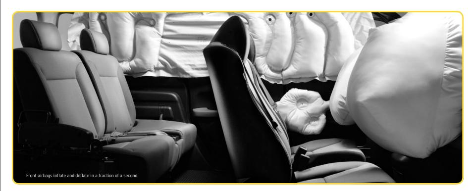
No less than six airbags stand ready to help protect Element occupants in sufficient impacts. The array includes dual-stage, dual-threshold front airbags, front side airbags and side curtain airbags–all standard.\* \*Honda reminds you and your passengers to always buckle up. Children 12 and under are safest when properly restrained in the rear seat.
