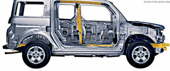
**Unit-body construction.** Incorporating front and rear crumple zones, the Element's chassis is designed to minimize the amount of crash energy entering the passenger compartment. Side-impact door beams help provide enhanced structural protection and help reduce the likelihood of cabin intrusion.
