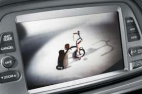
On navigation system-equipped models, the navigation screen doubles as a display for the innovative, full-color rearview camera. When you shift into reverse, the screen offers a clear view of the area immediately behind the vehicle. Parking sensors on Touring models also help keep you more aware of your space.
