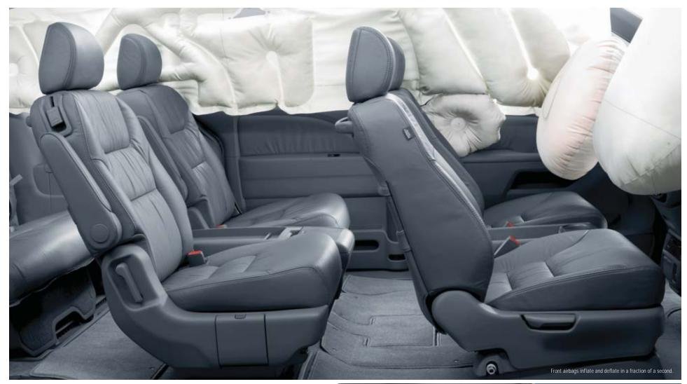
Front airbags,<sup>\*</sup> front side airbags and 3-row side curtain airbags with rollover sensor are standard. The dual-stage, dual-threshold front airbags deploy at one of two rates and thresholds depending on the severity of impact and seat-belt use. The Occupant Position Detection System (OPDS) helps prevent deployment of the passenger's side airbag if a child or small adult is in the airbag's deployment path.
