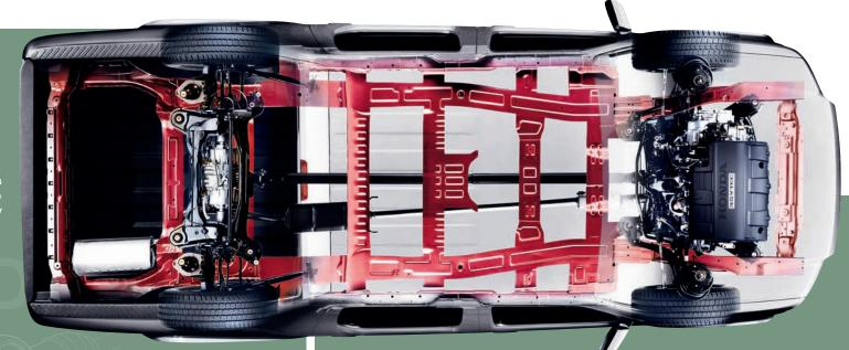
Like most 4-wheel-drive systems, the Ridgeline responds reactively to wheel slippage, sending power where it's needed most. But unlike competing systems, it also responds proactively based on the amount of torque the engine is producing. By anticipating the need to send power to additional traction points, it ensures a smooth and almost transparent transition between 2- and 4-wheel drive.
