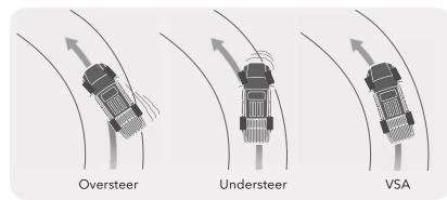
Vehicle Stability Assist™ (VSA®)† with traction control can detect oversteer or understeer and reduce the amount of engine torque and/or use the vehicle's ABS system to brake individual wheels as needed to help restore your intended course.
