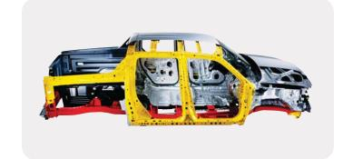
The Ridgeline's first line of defense is a reinforced unit body that incorporates a closed-box frame with internal high-strength steel frame stiffeners. Both the frame rails and all seven crossmembers feature box-section construction. The result is a remarkably high torsional rigidity.
