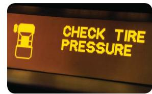
The Ridgeline's standard Tire Pressure Monitoring System (TPMS)<sup>5</sup> continually checks the pressure of each tire, alerting the driver with an in-dash display when a particular tire's pressure is significantly low.
