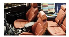
**SMARTER SEATING** Santa Fe Sport and GLS adapt to cargo or kids with just a flip of its 40/20/40 split-fold second row seats. An available sliding function adds even more versatility when you need to make room for an additional passenger or skis and snowboards.
