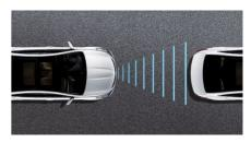
**FORWARD THINKING** Azera Limited comes standard with Forward Collision Warning. A forward-sensing camera looks down the road to determine the closing speed of your vehicle in relation to the vehicle ahead, and provides both audible and visual warnings to alert the driver of a potential collision.<sup>3</sup>
