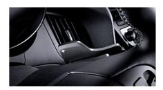
PADDLE SHIFT PRECISION Genesis Coupe's available 8-speed SHIFTRONIC automatic transmission features paddle shifters with revmatching to keep the engine's power band in the right place while approaching the cornering apex.
