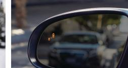
Forward Collision-Avoidance Assist Blind-Spot Collision Warning
