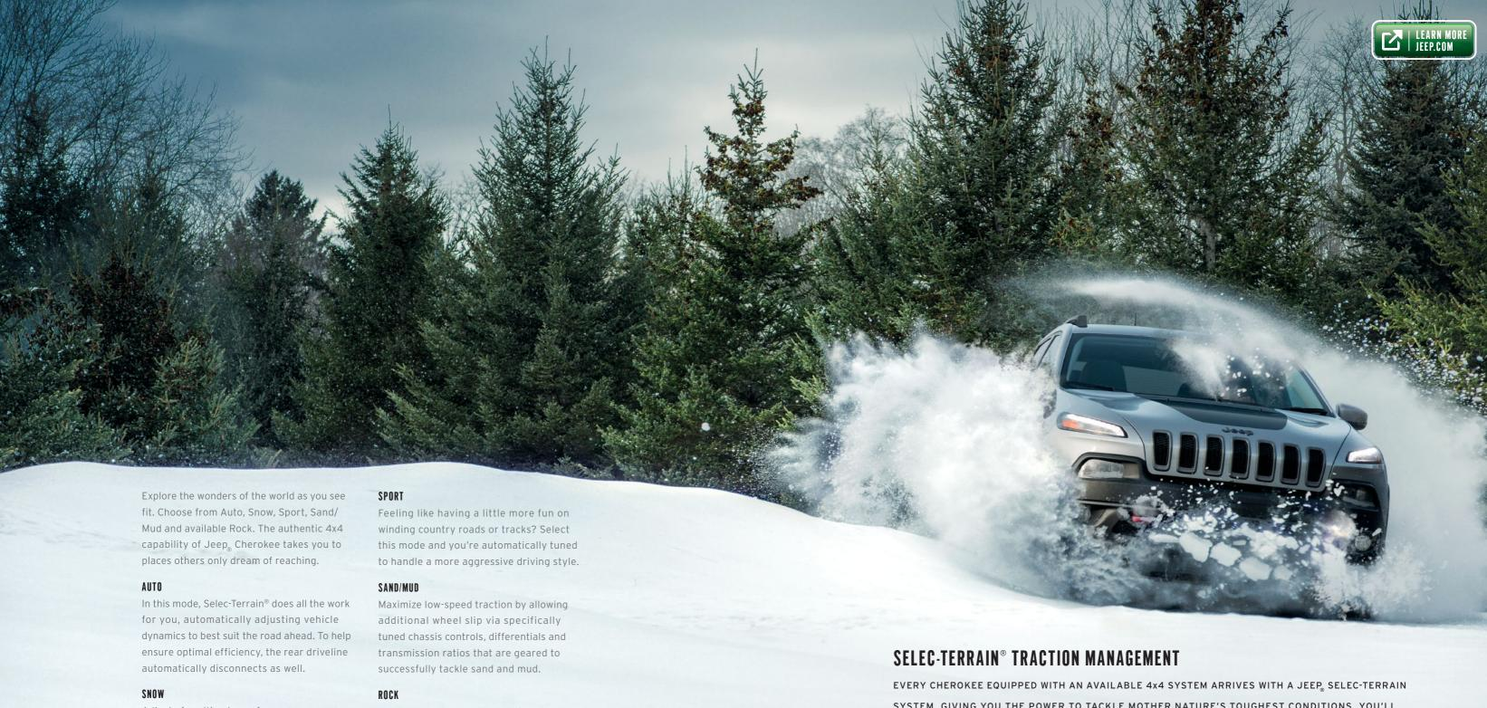
Adjusts for ultimate performance over snow- and ice-covered roads by maximizing vehicle stability and minimizing oversteer. Major systems auto-engaged and managed in this mode include antilock brakes and traction control.
