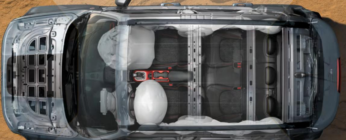
seven standard AIR BAGS<sup>4</sup> Your sense of security is met with this all-around air bag<sup>4</sup> system. Full-length front and rear side-curtain, driver inflatable knee bolster, seat-mounted side for front occupants, and advanced multistage driver and front-passenger air bags<sup>4</sup> all work together to help provide encompassing protection. Standard.
